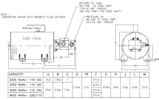
\* SUBTRACT 1 1/4" FROM OVERALL LENGTH FOR GENERATORS WITHOUT A FLOW DIVIDER (BCH SERIES) \*\* ADD 5/16" TO OVERALL HEIGHT FOR SHOCK MOUNTING WASHERS.
